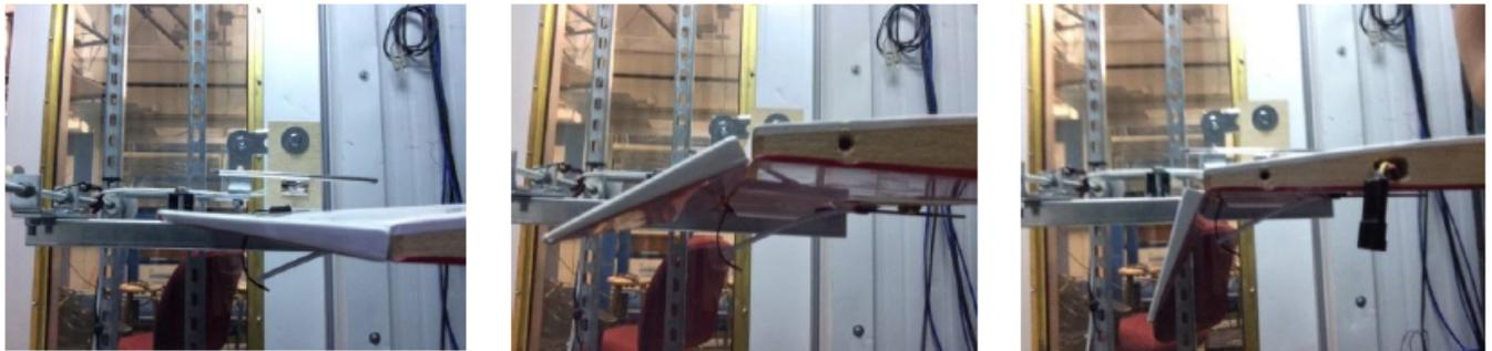
**Figure 10:** Aileron positions, (a) no deflection, (b) half deflection, and (c) full deflection.
