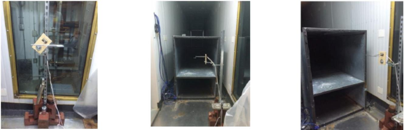
Figure 5: Test setup for AOA sensors in the wind tunnel with no wing.
