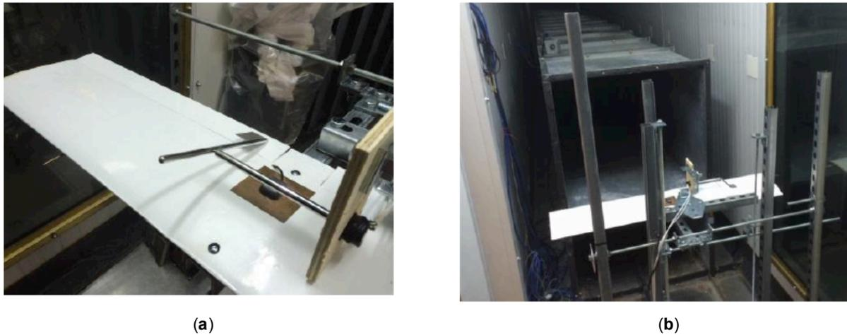
Figure 7: Setup for large AOA sensor located on the upper surface of the wing: (a) wing and sensor, (b) wind tunnel test section and wing fixed on a stand.
