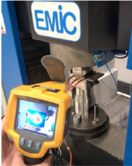
Figure 4: Fluke Ti10 thermographic camera used for thermal monitoring of the die–specimen–punch assembly during testing.
