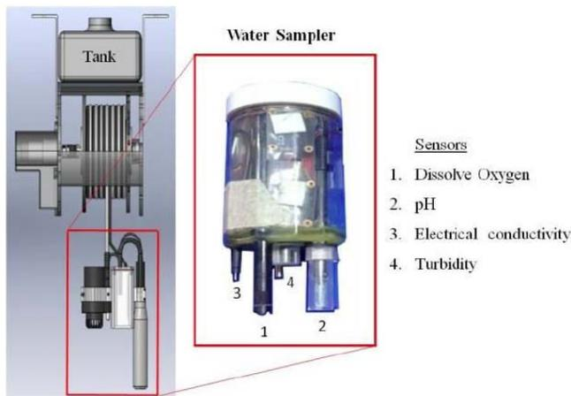
**Figure 5:** Typical payload system of UAAV.
