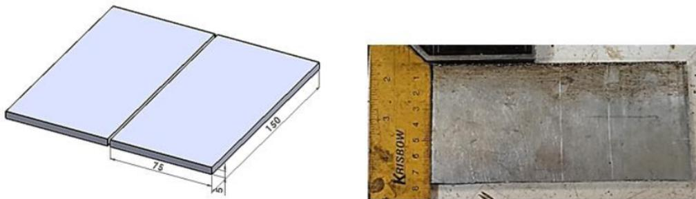
**Figure 1: Dimensions of Aluminum AA5052 Materials.**
