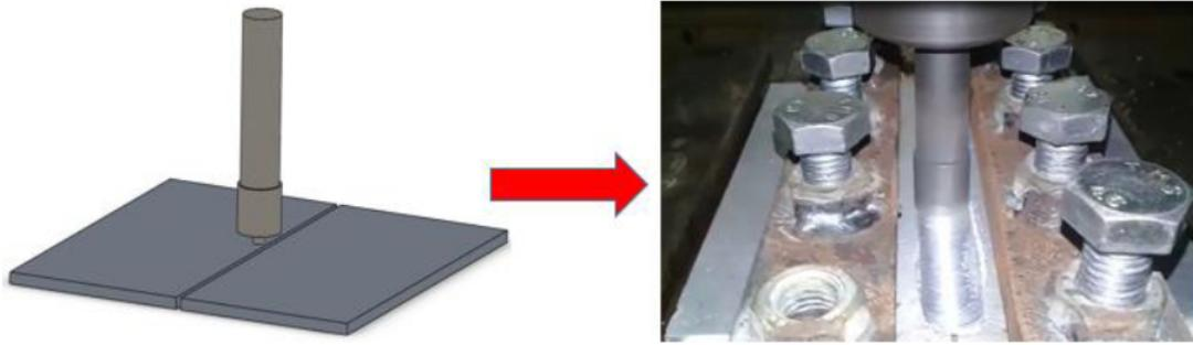
**Figure 3:** Friction Stir Welding Schematic.
