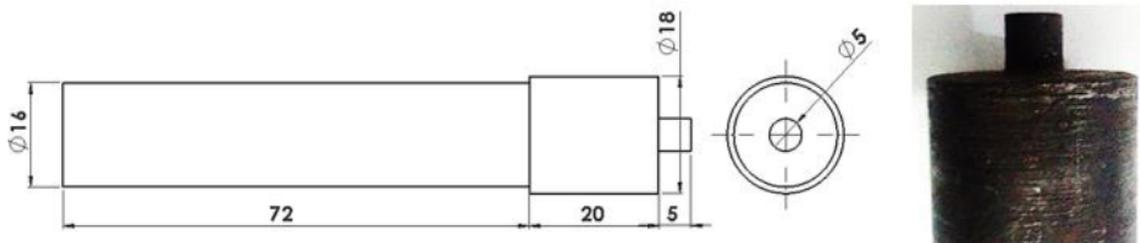
**Figure 2: Pin designs and profiles.**
