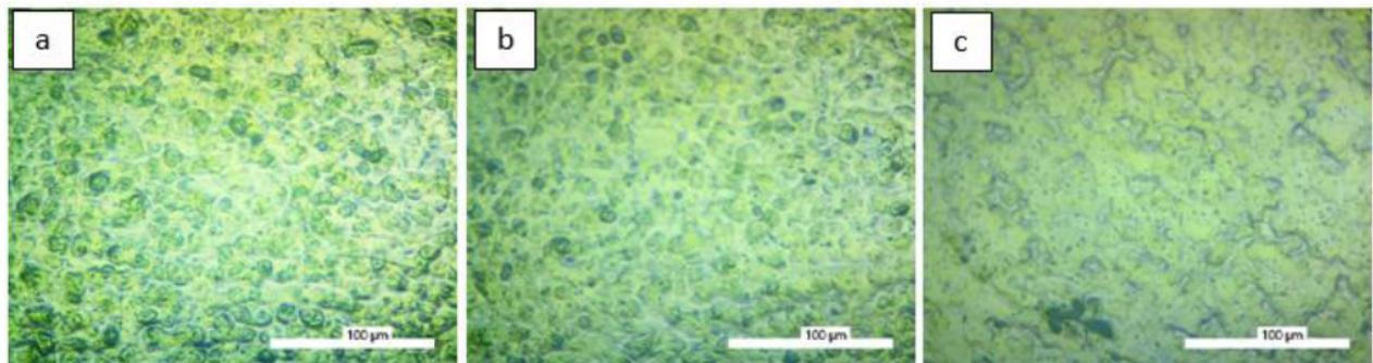
**Figure 9:** TMAZ Microstructure, a) 1000 rpm, b). 1200 rpm, c). 1500 rpm.
