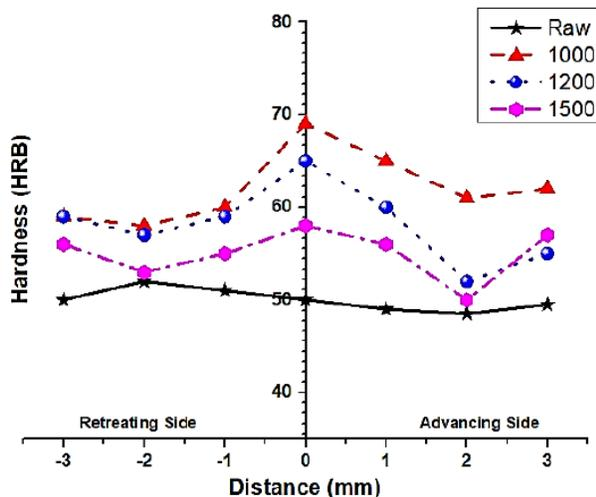
Figure 12: Rockwell Hardness.
