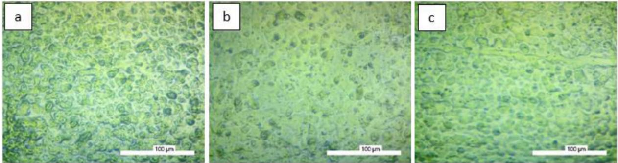
**Figure 8:** HAZ Microstructure, a). 1000 rpm, b). 1200 rpm, c). 1500 rpm.
