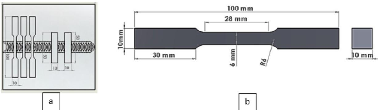
**Figure 4:** a). Sample area, b). Tensile Testing Specimen Standard (ASTM E8M).
