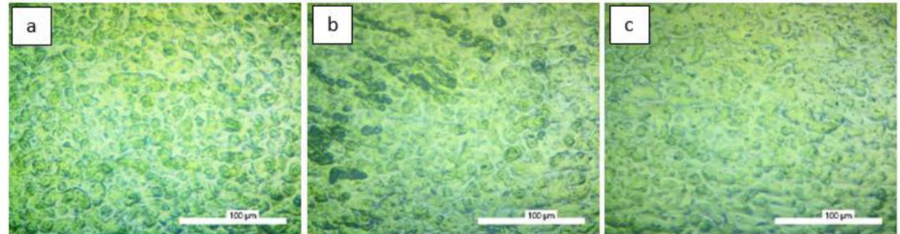
**Figure 10:** Weld Nugget Microstructure, a). 1000 rpm, b). 1200 rpm, c). 1500 rpm.
