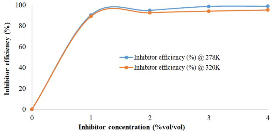
**Figure 4:** Inhibitor efficiency and varied concentrations of the inhibitor at different temperatures.
